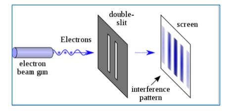
A beam of electrons pass through a first screen with two slits and impinges on a final screen where electrons are absorbed.
